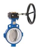
Valves of all sizes can be direct mounted with gear operators for manual operation. Gear operators can also be attached with chain-wheel operators to open or close valves located on pipelines at high elevations.
